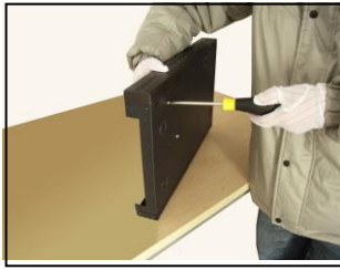
④fix the screw of hard disk
