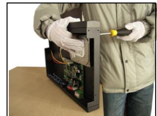
③fix the screw of hard disk
