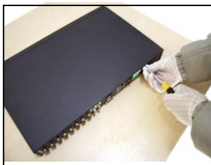
① disassemble the screw
