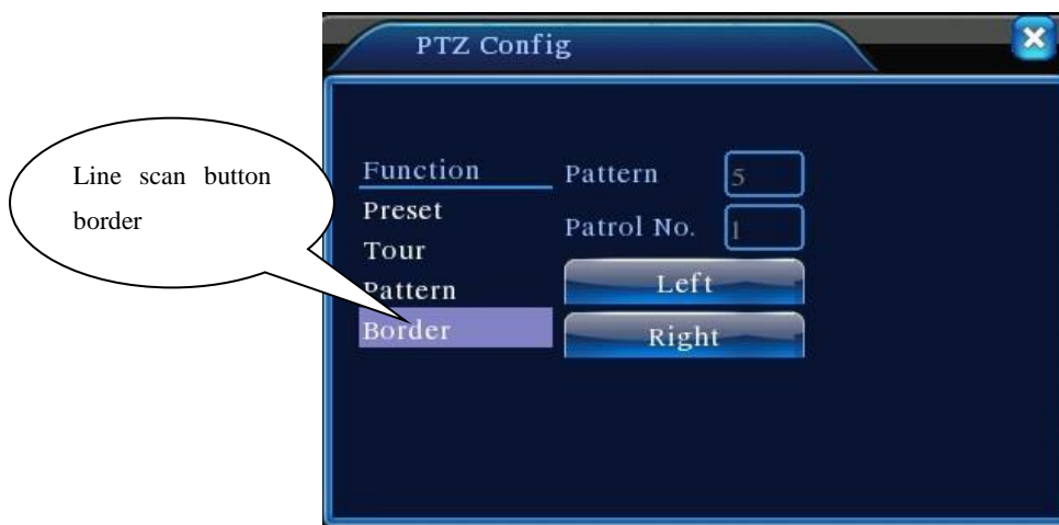
Picture 3.15 Boundary Scan Setup
