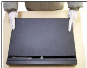
②disassemble the cover
