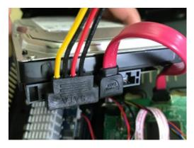
Connect the other side of the hard disk data cable and power cable to the hard disk.
