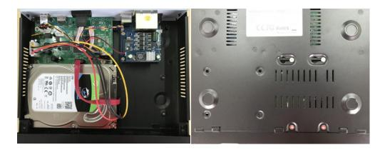
Align the screw holes on the hard disk with the screw holes on the chassis of the box and screw them one by one.
