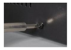
Screw the back panel and side of the boot box, then remove the cover plate.
